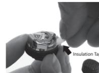
Pull and remove Insulation Tab from AROFLY to connect battery. Replace the cap to AROFLY.
