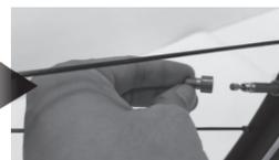
Install "Valve Adaptor" on Presta valve. Ensure the correct side of the Adaptor to the Valve.
