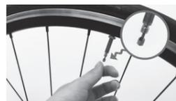
If it is a Presta valve, please loosen "the valve pin" to the top-end of the Presta valve shaft.
