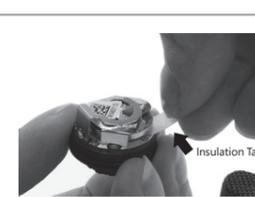
Pull and remove Insulation Tab from AROFLY to connect battery. Replace the cap to AROFLY.
